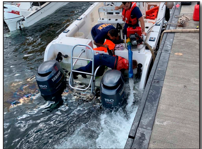
Figure 35-62 Dewatering operations are an important consideration the IC must begin to coordinate early on with the assistance of Lifeguards, Harbor PD, and/or USCG
