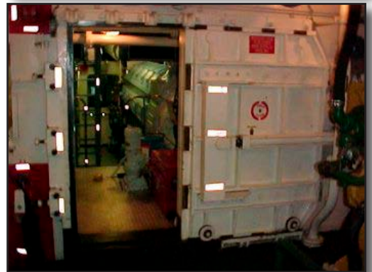
Figure 35-39 Remote controlled automatic watertight door
