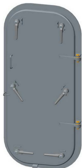
Figure 35-38 Individually Dogged watertight door
