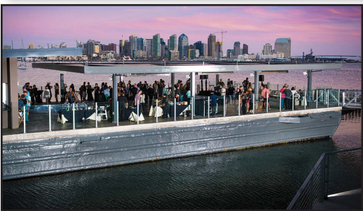
Figure 35-33 Museum ships (top) and Coastera restaurant both fall under the classification of floating structures and are not inspected by the USCG.
