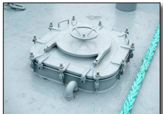
Figure 35-41 Access Hatch (Scuttle)
